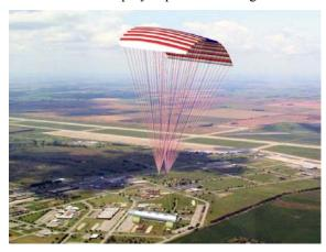
Under the action of aerodynamic forces, the booster reenters in a controlled, slow flat spin effectively slowing the descent via aerobraking, its velocity being reduced, with the assistance of a deployed drogue, to the sub-sonic at about 20,000 feet. A parafoil is subsequently deployed to slow its descent and provide a relatively horizontal glide back to the launch site for landing using a set of deployed pressurized bags.
