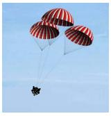
splash down at an estimated rate of 25 km/hr (15.5 mph). Inflatable bags around the perimeter base will soften the landing and will keep the vehicle afloat should it land on water.
