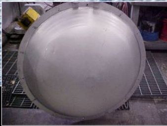
Structures & Materials: Developing friction stir welding and spin forming manufacturing processes for Ares I Upper Stage propellant tanks.
