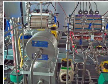
Energy Storage: Regenerative fuel cells to store energy during the lunar night.
