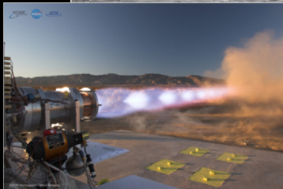
Propulsion & Cryogenics: Prototype LOX-Methane engine for ascent stage
